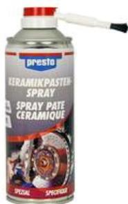
Metal-free high-temperature paste with excellent lubricating effect. Good corrosion protection. Ideally suited for assembly work on ABS brake systems as well as for long-term lubrication of highly loaded sliding surfaces of all kinds. Temperature resistant from -40 ° C to + 1,400 ° C. The removable brush head allows for easy even application of the paste.
