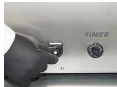
Step 14: Switch-on the machine. The solvent is cleaning the pump from eventually residues coming from manufacturing. Afterwards take out the cleansing can and begin with the real filling process.
