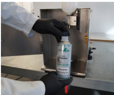
Step 9: Before filling the machine has to be rinsed with solvent. For it take off the screw plug of the cleansing can...
