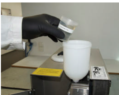
Step 12: Pour 100 ml solvent into the opened gravity feed cup.
