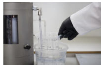
**Step 4:** Close the door and take under the second hose a collecting tray for the contaminated solvent. Insert the hose.
