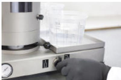
**Step 5:** Turn the switch to „suction“. The solvent will be sucked.
