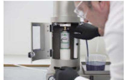
**Step 5:** Set a 150 ml spray can on the distance adapter. In doing so place the can valve exactly under the filler neck and lock it with the lever.
