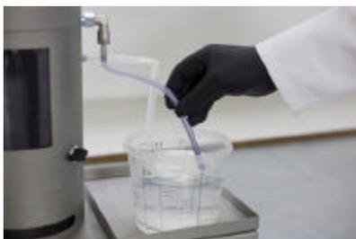
**Step 1:** Instead of the varnish container put a container with the filled lacquer suitable solvent under the suction hose.
