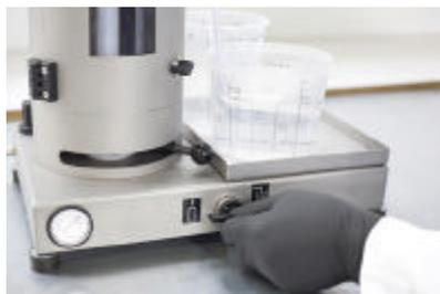
**Step 6:** Then switch to position „filling“. Because the filling is blocked, the contaminated solvent will be conducted into the collecting tray.
