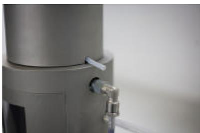
**Info:** As soon as a varnish drop is coming out of the pictured hose an impervious core is damaged and must be replaced. For it send the machine to the manufacturer.
