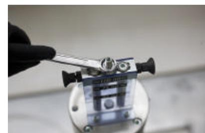
**Step 8:** A vernier adjustment is possible with a screw-wrench no. 17.
