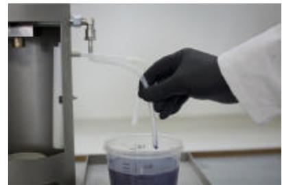
**Step 2:** Put the container with varnish on the bin and insert the suction hose.
