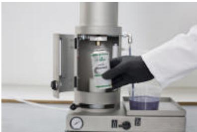
**Step 12:** Open the door, take out spray can. The filling machine is now ready to fill more spray cans with the same lacquer.
