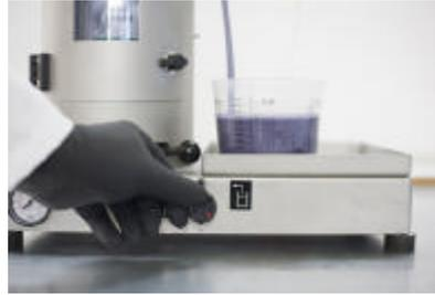
**Step 10:** Turn the switch to „suction“ – the colour will be drawn into the machine. Depending on the viscosity of the lacquer takes it more time.
