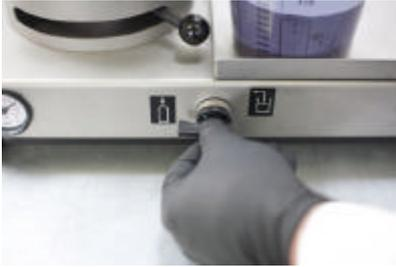
**Step 9:** With the switch on the front you can choose either the position „suction“ (on the right) or „filling“ (on the left).
